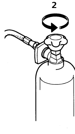
Fig. 31 Filling the compressed air cylinders
