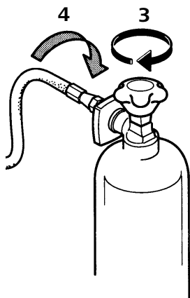
Fig. 32 Removing the compressed air cylinders
